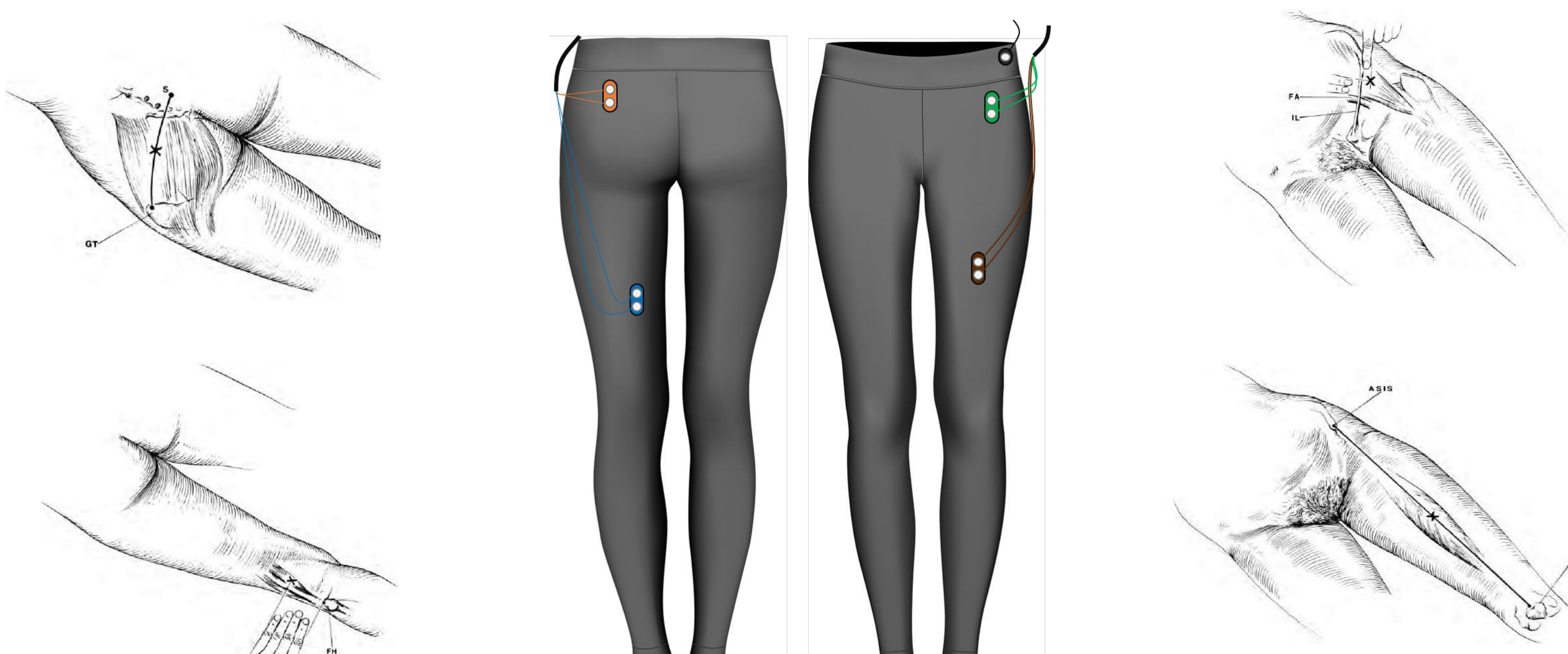
Fig. 4 Leggings with electrodes and the main muscles at which the electrodes are aimed to read.
